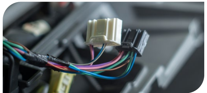
Rynite® is used for automotive and electrical applications such as automotive connectors due to its electrical insulation, high temperature resistance and mechanical properties.
