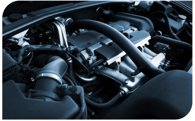
Zytel® is used to reduce weight and cost by replacing metal in many automotive applications, including engine covers.
