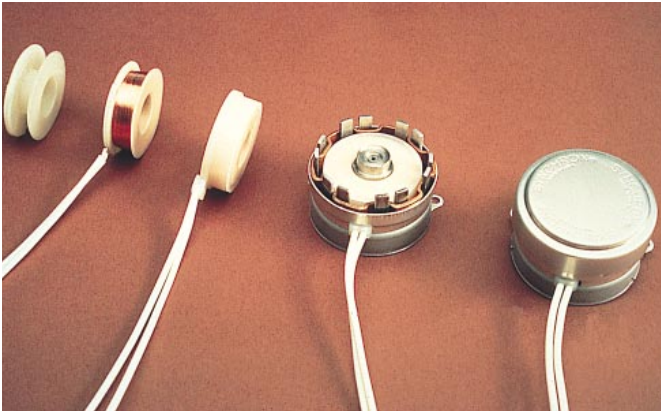
Fig. 34. Encapsulated stator coil replaces a tape-insulated unit in a hysteresis synchronous motor that operates timing devices, vents, and valves in heating, ventilation, and air conditioning equipment. Both coil bobbins and encapsulation are in ZYTEL® PA66. Encapsulated coils withstand 3000 V versus a test limit of 2200 V for the taped coils being replaced (Hansen Corp.).
