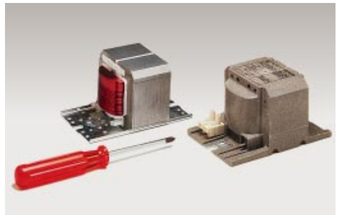
Fig. 41. Philips lighting choke transformers (250 and 400 W) for gas discharge lighting encapsulated in RYNITE® 935, a PET polyester with glass and mineral reinforcement.
