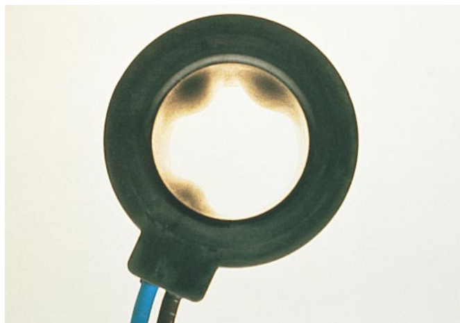
Fig. 17. Result of encapsulating a wound coil bobbin that is not fully crystallized.
