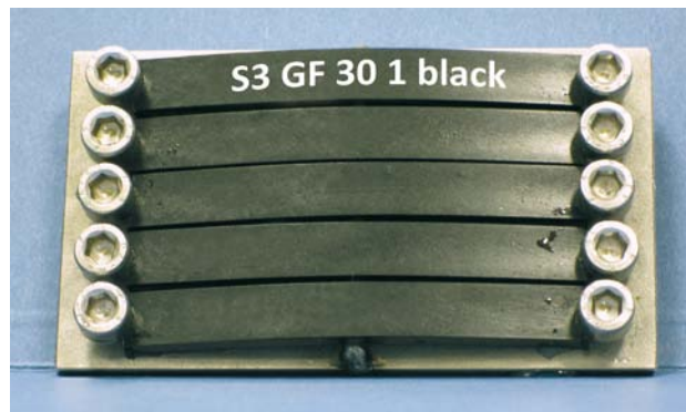
AKROMID® S3 GF 30 1 following ageing in ZnCl 2 solution under flexural load
